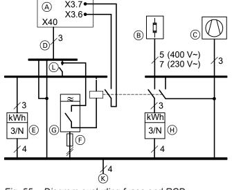
Fig. 55 Diagram excluding fuses and RCD
