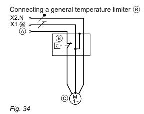
Connecting the temperature limiter, part no. 7151728, 7151729  $^{\circ}$
