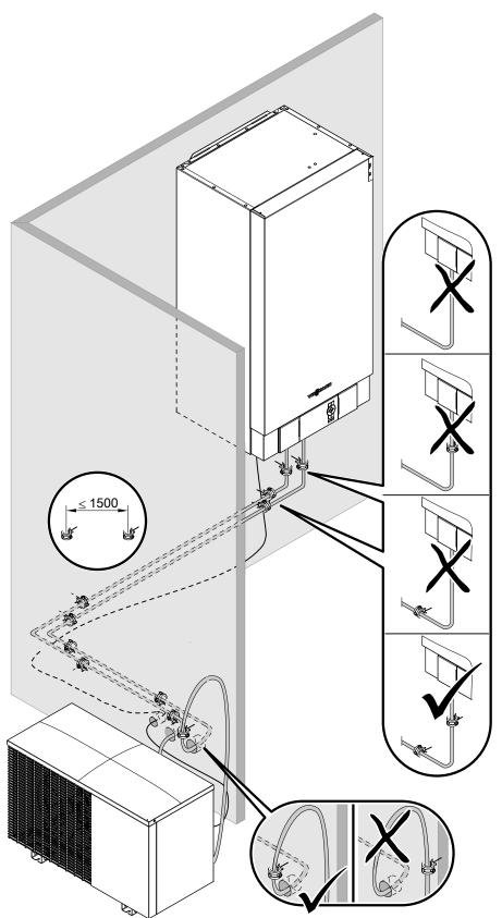
Fig. 26 Pipe bend for vibration compensation outside the building
