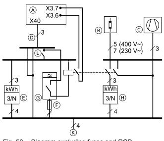
Fig. 58 Diagram excluding fuses and RCD
