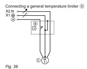
Connecting the temperature limiter, part no. 7151728, 7151729 ® X2 N
