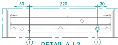
DETAIL A 1:3 WALL FIXATION
