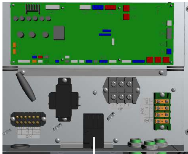
a Booster heater contactor K3M
