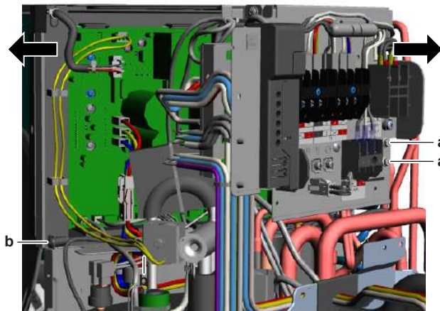
a Screw (wire terminal mounting plate) b Screw (switch box)
